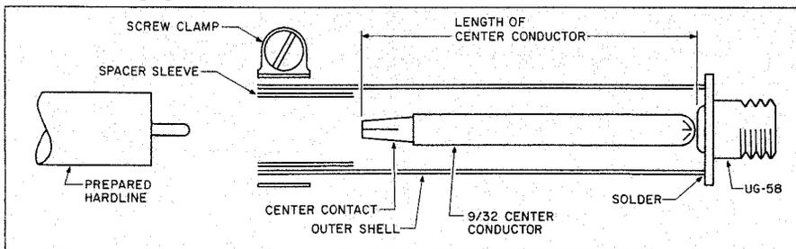
Figure 1. Cutaway of  $1/4$  wave impedance converter, showing all parts of the completed unit.
